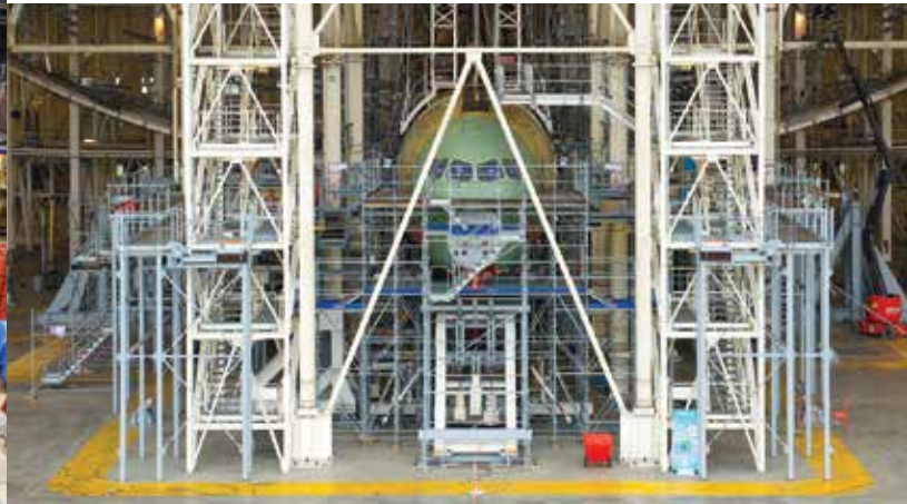
Toulouse: scaffolding for Airbus A350-900 resistance tests.
